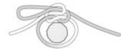
Quick release knot to secure seaweed to lines. Knots released by pulling single loop end.
