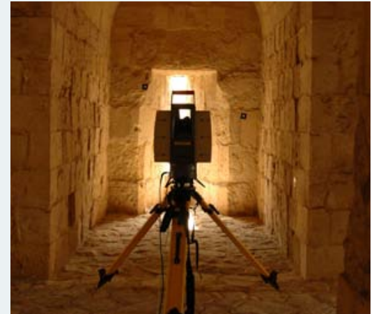
Leica 3D scanner inside the Bab al-Barqiyya, Al-Azhar Park, Cairo, Egypt
